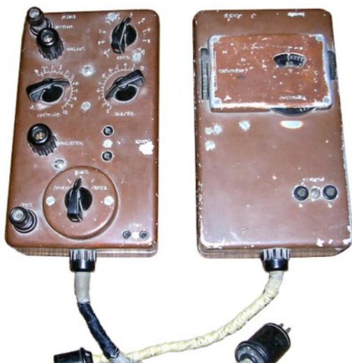
Later found photos of a well used Morava transmitter unit (left) and receiver unit (right). The metal case with the interface box and Morse key appeared to be missing. (Source of photo not yet identified.)
